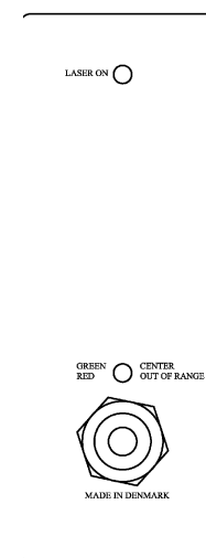
Fig. 3 Light indicators for laser (emission) on and measurement at centre or out of range
