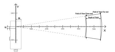
Standard Models of the O2DS scanner can be delivered in 8 different measuring ranges, and each in two versions with different measuring angles, either 10° or 50° and then in 2 or 3 scan rates giving high or low angular resolution, and can furthermore be customized to other than standard scan angels and measuring ranges.
